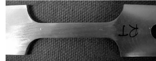
As welded specimen
